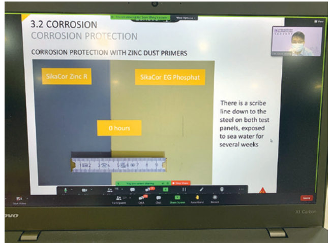
Sean explains the corrosion protection technique commonly adopted by the construction industry.
