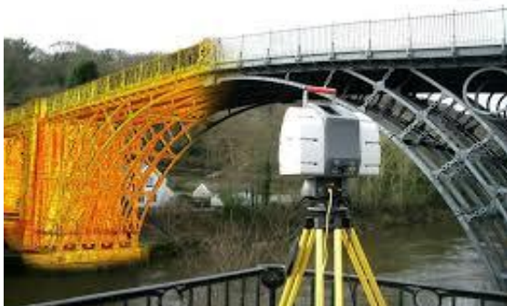
Static Laser scanner
