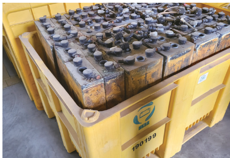
Disused Lead Acid Batteries for Recycling
