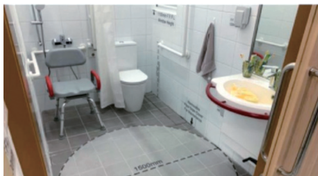
Accessible and Adaptable Design Bathroom
