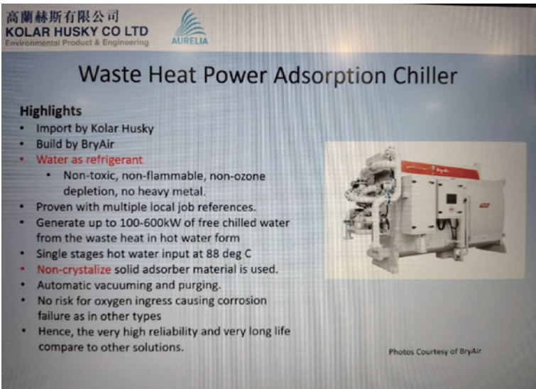
Figure 2: Waste Heat Power Absorption Chiller
