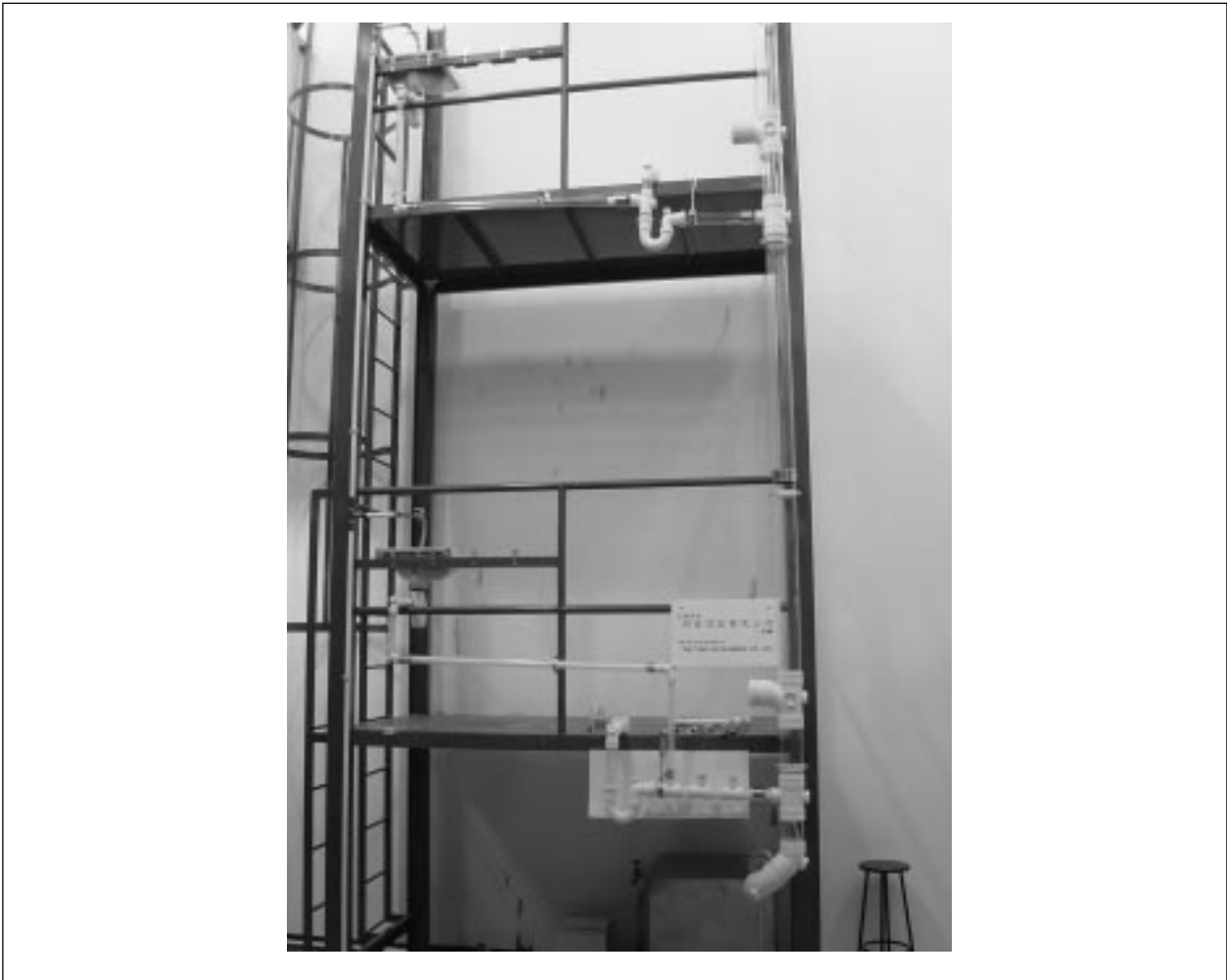
Figure 3 A full-scale drainage test rig. The drainage configuration that was proposed by the HKIE (2003) is shown at the upper storey of the setup. The Back-filling drainage configuration as proposed by Yuen et al. (2003) was installed at the lower storey of the test rig.
